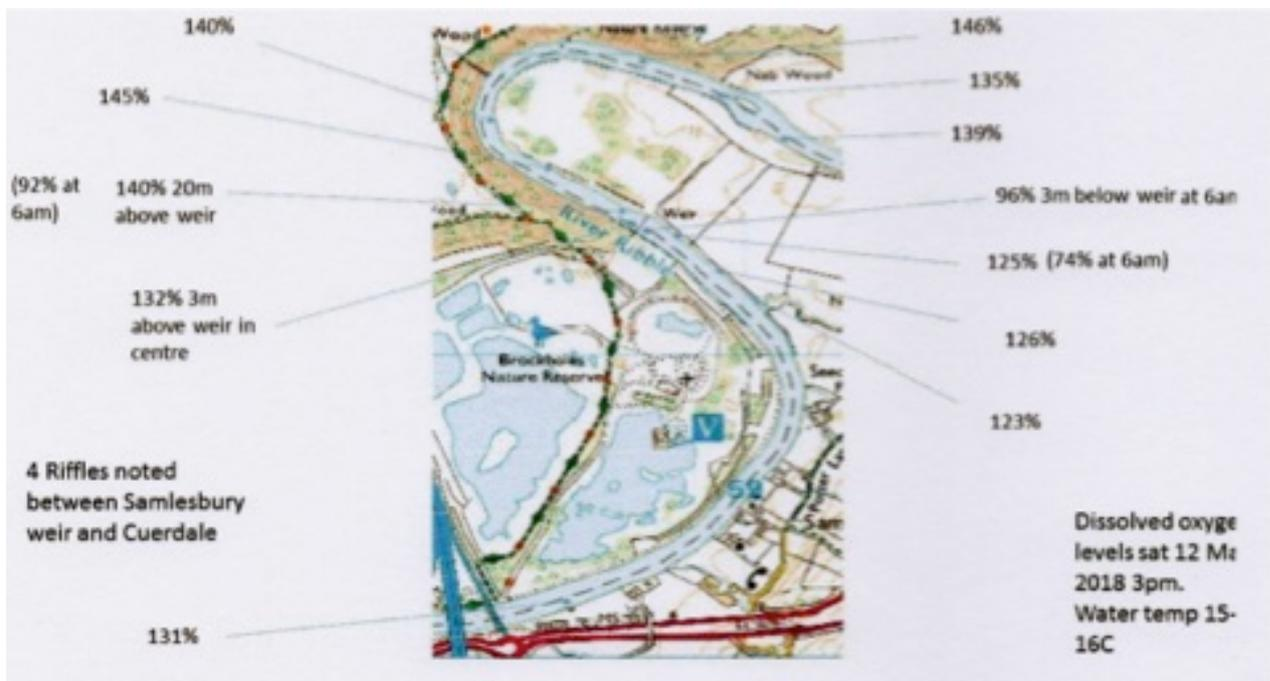
**NOTE- Calibration of the probe is carried out in air (which sets the probe at 100%. Deviations above or below 100% are recorded as shown on the diagram above.**
